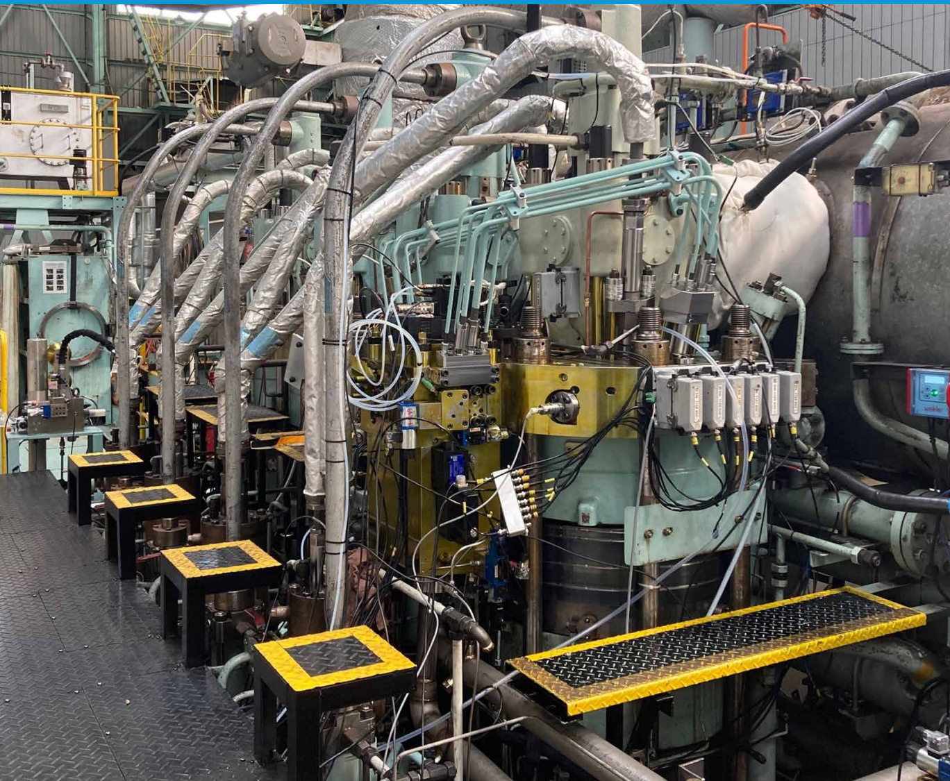
Hydrogen combustion test on 4S50ME-T
